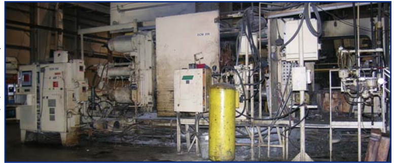
PRINCE MODEL 1651 1600-TON CAPACITY, COLD CHAMBER ALUMINUM DIE CASTING MACHINE
